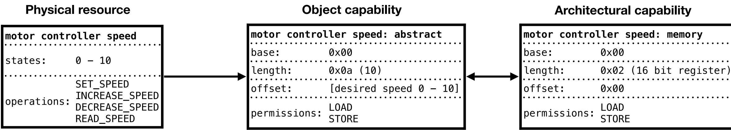
Motor controllers convert an intuitive input (e.g., relative speed 0 to 10) to the motor's actual control mechanism (e.g., frequency)
