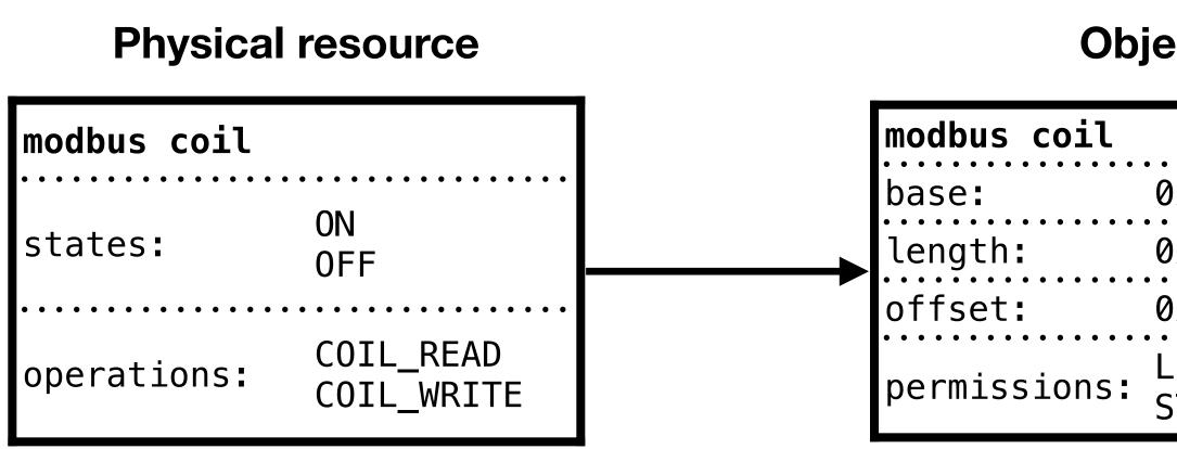
A coil is an object that can be energised or deenergised at a given voltage to control solenoids, energise motors, trip breakers, etc.
